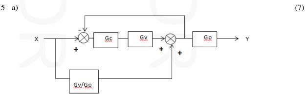
Determine the transfer function Y(s)/X(s) for the block diagrams shown above. Express the result in terms of Gc, Gv and Gp.
