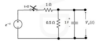
b) Determine current flowing through the circuit shown for  $t \ge 0$
