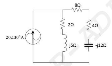
10 a) State reciprocity theorem. Verify reciprocity theorem for the circuit given (5) below.
