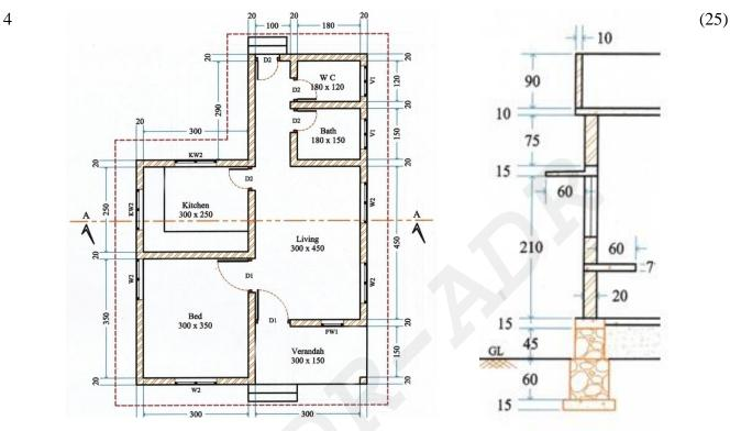
Prepare a detailed estimate of the following items (a) Earth work excavation, Width of base Concrete 75cm (b) Foundation (60cm x 60cm) and basement (45cm x 45xm) with RR masonry (c) Brick work for super structures, CM1:6 (d) RCC work for roof and sunshade (e) Wood work for door frame and shutters of door and windows (Door D1 -100x210; D2 -80x210; W2 -120x140; V1- 90x60; KW2- 120x90; FW1- 60x180) All dimensions are in centimeters. (Any missing data may be suitably assumed)
