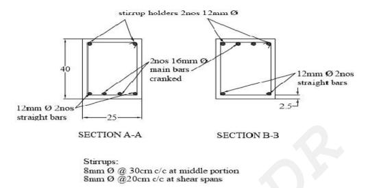
Prepare a bar bending schedule of the simply supported beam of size 25cm x 40cm shown in the figure. (All dimensions are in Centimetres)
