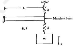
Take L = 3m. EI for beam = 27 Nm<sup>2</sup>, stiffness for each spring, k = 3 N/m and mass m = 3 kg
